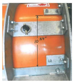
1. Install two Poly Wing Brackets 53286-A-GA as shown on the picture above. Using c-clamp clamp the Poly Wing Brackets 53286-A-GA to the rib of the blade. Using holes in
